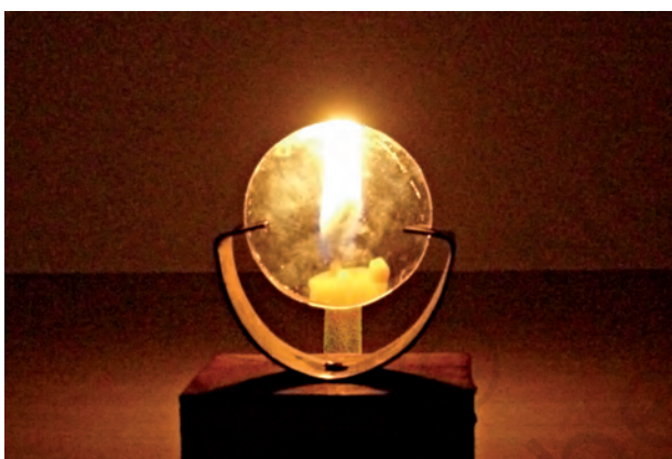
Fig. 15.26 Virtual image formed by the convex lens
