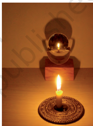
Fig. 15.19 Image formed by a convex mirror
