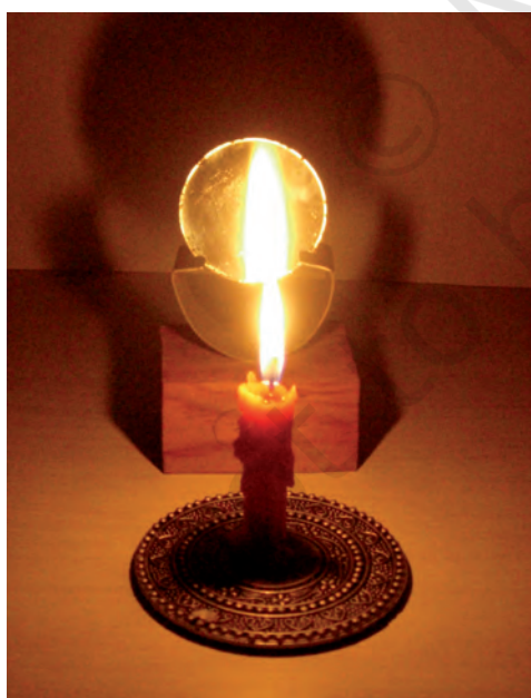
Fig. 15.16 Virtual image formed by a concave mirror
