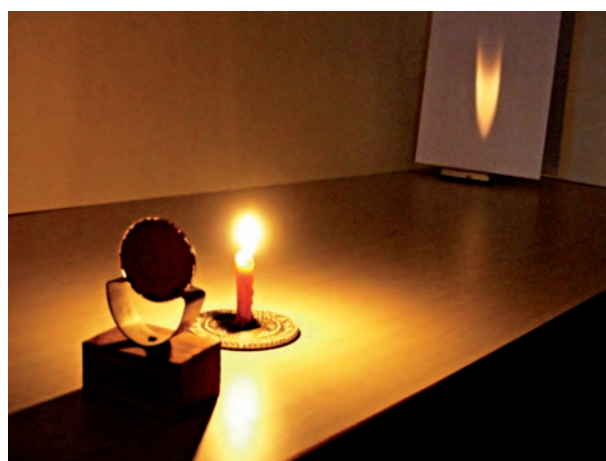
Fig. 15.15 Real images formed by a concave mirror
