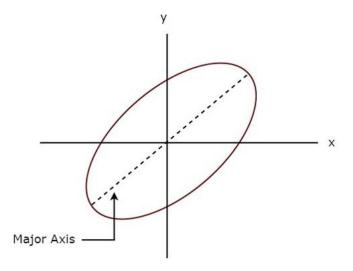
The above Lissajous figure is in **elliptical shape** and its major axis has some inclination angle with positive x-axis.
