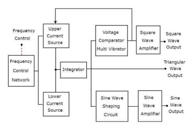
There are two **current sources**, namely upper current source and lower current source in above block diagram. These two current sources are regulated by the frequency-controlled voltage.
