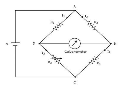
In above circuit, the arms AB, BC, CD and DA together form a **rhombus** or square shape. They consist of resistors  $R_2$ ,  $R_4$ ,  $R_3$  and  $R_1$  respectively. Let the current flowing through these resistor arms is  $I_2$ ,  $I_4$ ,  $I_3$  and  $I_1$  respectively and the directions of these currents are shown in the figure.
