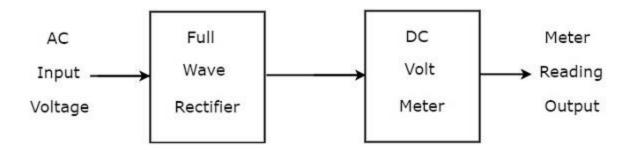
The above block diagram consists of two blocks: full wave rectifier and DC voltmeter. We will get the corresponding circuit diagram just by replacing each block with the respective component(s) in above block diagram.
