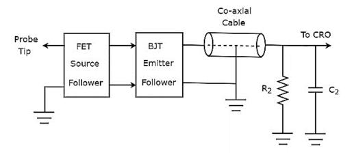
As shown in the figure, the probe head consists of a FET source follower in cascade with BJT emitter follower. The FET source follower provides high input impedance and low output impedance. Whereas, the purpose of BJT emitter follower is that it avoids or eliminates the impedance mismatching.
