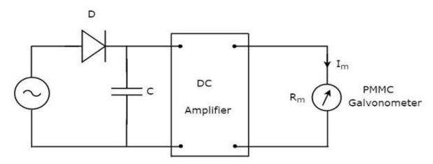
The above circuit consists of a diode, capacitor, DC amplifier and PMMC galvanometer. The diode present in the above circuit is used for **rectification** purpose. So, the diode converts AC voltage signal into a DC voltage signal. The capacitor charges to the peak value of this DC voltage signal.
