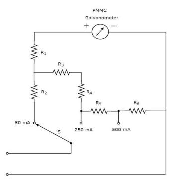
The above circuit looks like a multi range DC ammeter. the combination of a resistor in parallel with PMMC galvanometer is a **DC ammeter**. So, it can be used to measure DC currents up to certain value.
