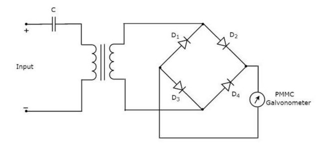
This basic wave analyzer can be used for analyzing each and every harmonic frequency component of a periodic signal.
