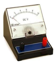
The DC voltmeter shown in above figure is a (0-10)V **DC voltmeter**. Hence, it can be used to measure the DC voltages from zero volts to 10 volts.
