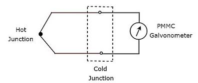
The part of the circuit, which lies between hot & cold junctions including those two junctions is an equivalent model of basic thermocouple. A PMMC galvanometer is connected across the cold junction and it deflects according to the emf generated across cold junction. **Thermocouple transducer** is the most commonly used thermoelectric transducer.
