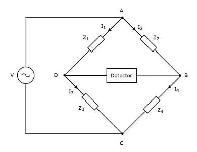
As shown in above figure, AC bridge mainly consists of four arms, which are connected in rhombus or **square shape**. All these arms consist of some impedance.
