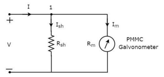
We have to place this **DC ammeter** in series with the branch of an electric circuit, where the DC current is to be measured.
