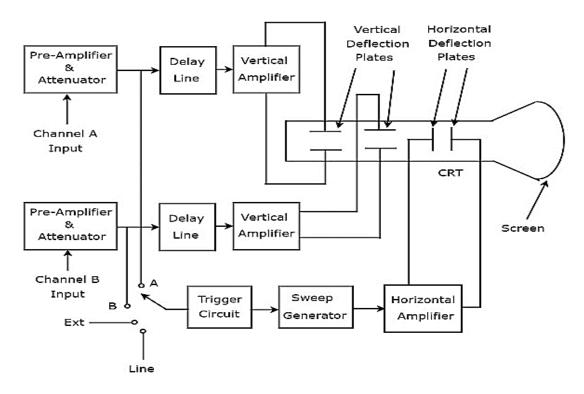
As shown in above figure, the CRT of Dual Beam Oscilloscope consists of two sets of vertical deflection plates and one set of horizontal deflection plates.
