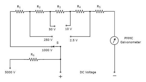
The above circuit looks like a multi range DC voltmeter. The combination of a resistor in series with PMMC galvanometer is a **DC voltmeter**. So, it can be used to measure DC voltages up to certain value.
