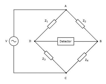
The circuit diagram of AC bridge is similar to that of DC bridge. The above AC bridge has **four arms** and each arm consists of some impedance. That means, each arm will be having either single or combination of passive elements such as resistor, inductor and capacitor.
