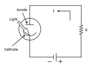
The **working** of photo electric transducer is mentioned below.
