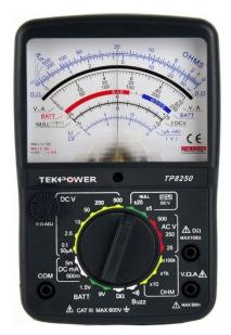
As shown in the figure, this multimeter can be used to measure various high resistances, low resistances, DC voltages, AC voltages, DC currents, & AC currents. Different scales and range of values for each of these quantities are marked in above figure.
