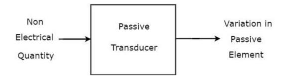
As shown in the figure, passive transducer will produce variation in the passive element in accordance with the variation in the non-electrical input quantity (or signal).
