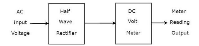
The above block diagram consists of two blocks: half wave rectifier and DC voltmeter. We will get the corresponding circuit diagram, just by replacing each block with the respective component(s) in above block diagram. So, the **circuit diagram** of AC voltmeter using Half wave rectifier will look like as shown in below figure.
