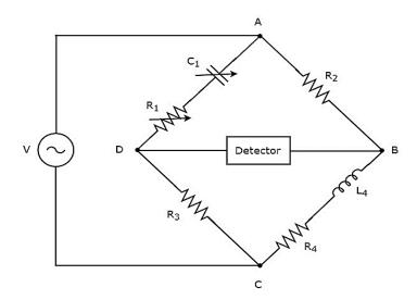
In above circuit, the arms AB, BC, CD and DA together form a rhombus or square shape. The arms, AB and CD consist of resistors,  $R_2$  and  $R_3$  respectively. The arm, BC consists of a series combination of resistor,  $R_4$  and inductor,  $L_4$ . The arm, DA consists of a series combination of resistor,  $R_1$  and capacitor,  $C_1$ .
