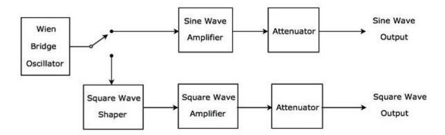
The above block diagram consists of mainly **two paths**. Those are upper path and lower path. Upper path is used to produce AF sine wave and the lower path is used to produce AF square wave.
