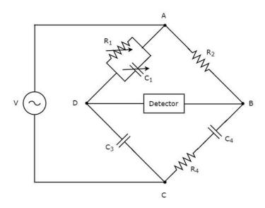
In above circuit, the arms AB, BC, CD and DA together form a rhombus or **square shape**. The arm AB consists of a resistor,  $R_2$ . The arm BC consists of a series
