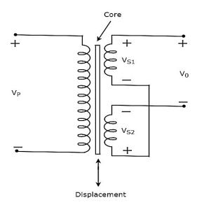
The transformer present in above circuit has a primary winding and two secondary windings. Here, the ending points of two secondary windings are joined together. So, we can say that these two secondary windings are connected in **series opposition**.
