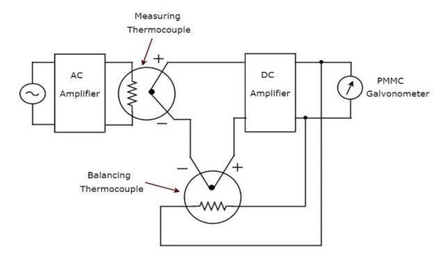
The above circuit consists of an AC amplifier, two thermocouples, DC amplifier and PMMC galvanometer. AC amplifier amplifies the AC voltage signal. Two thermocouples that are used in above circuit are a measuring thermocouple and a balancing thermocouple. **Measuring thermocouple** produces an output voltage, which is proportional to RMS value of the AC voltage signal.
