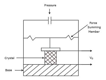
The **output voltage**,  $V_0$  of above pressure transducer will be
