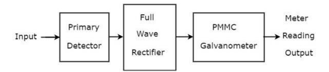
The **function** of each block present in basic wave analyzer is mentioned below.
