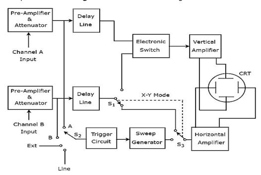
As shown in above figure, the CRT of Dual Trace Oscilloscope consists of a set of vertical deflection plates and another set of horizontal deflection plates. **channel** consists of four blocks, i.e. pre-Amplifier & attenuator, delay line, vertical amplifier and vertical deflection plates.
