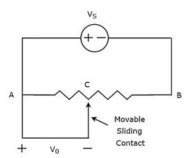
The above circuit consists of a potentiometer and a voltage source,  $V_S$ . We can say that these two are connected in parallel with respect to the points A & B. Potentiometer has a sliding contact, which can be varied. So, the point C is a variable one. In above circuit, the **output voltage**,  $V_0$  is measured across the points A & C.
