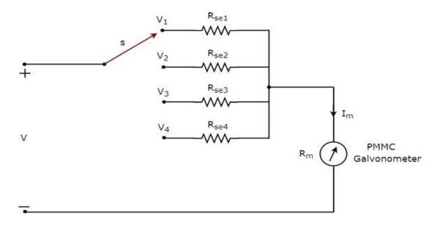
We have to place this **multi range DC voltmeter** across the two points of an electric circuit, where the DC voltage of required range is to be measured. We can choose the desired range of voltages by connecting the switch *s* to the respective multiplier resistor.
