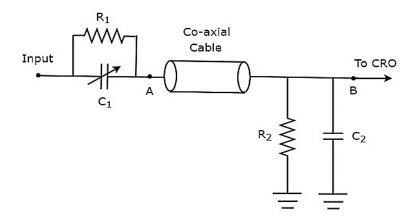
As shown in the figure, the probe head consists of a parallel combination of resistor,  $R_1$  and a variable capacitor,  $C_1$ . Similarly, the termination circuit consists of a parallel combination of resistor,  $R_2$  and capacitor,  $C_2$ .
