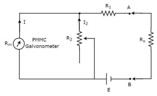
The part of the circuit, which is left side of the terminals A & B is **series ohmmeter**. So, we can measure the value of unknown resistance by placing it to the right side of terminals A & B. Now, let us discuss about the **calibration scale** of series ohmmeter.
