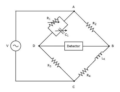
In above circuit, the arms AB, BC, CD and DA together form a rhombus or square shape. The arms AB and CD consist of resistors,  $R_2$  and  $R_3$  respectively. The arm, BC consists of a series combination of resistor,  $R_4$  and inductor,  $L_4$ . The arm, DA consists of a parallel combination of resistor,  $R_1$  and capacitor,  $C_1$ .
