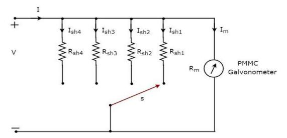
Place this multi range DC ammeter in series with the branch of an electric circuit, where the Direct Current of required range is to be measured. The desired range of currents is chosen by connecting the switch, s to the respective shunt resistor.
