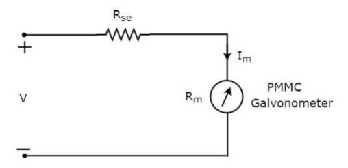
We have to place this DC voltmeter across the two points of an electric circuit, where the DC voltage is to be measured.
