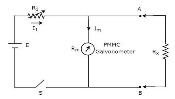
The part of the circuit, which is left side of the terminals A & B is **shunt ohmmeter**. So, we can measure the value of unknown resistance by placing it to the right side of terminals A & B.
