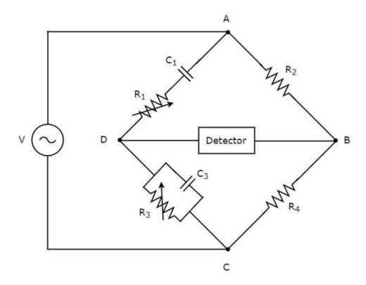
In above circuit, the arms AB, BC, CD and DA together form a rhombus or **square shape**. The arms, AB and BC consist of resistors,  $R_2$  and  $R_4$  respectively. The arm, CD consists of a parallel combination of resistor,  $R_3$  and capacitor,  $C_3$ . The arm, DA consists of a series combination of resistor,  $R_1$  and capacitor,  $C_1$ .
