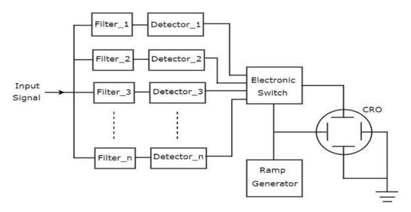
The **working** of filter bank spectrum analyzer is mentioned below.
