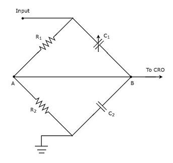
We can balance the bridge, by adjusting the value of variable capacitor,  $C_1$ . We will discuss the concept of bridges in the following chapters. For the time being, consider the following **balancing condition of AC bridge**.
