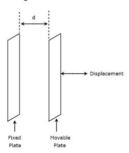
The **capacitor**, which is present in above circuit has two parallel plates. Among which, one plate is fixed and the other plate is a movable one. Due to this, the spacing between these two plates will also vary. the value of capacitance changes as the spacing between two plates of capacitor changes.
