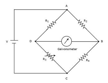
The above DC bridge has **four arms** and each arm consists of a resistor. Among which, two resistors have fixed resistance values, one resistor is a variable resistor and the other one has an unknown resistance value.
