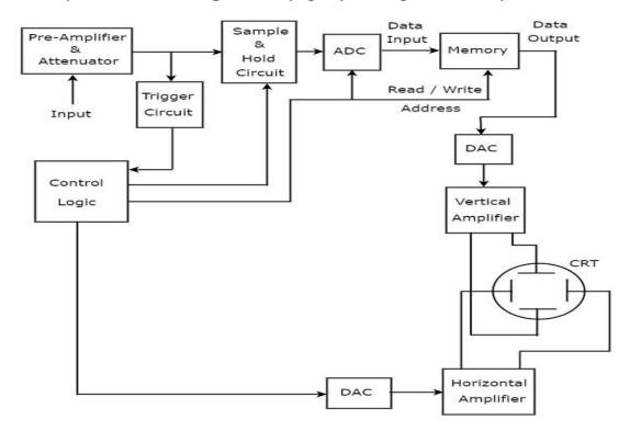
Additional blocks required for digital data storage are added to a basic oscilloscope to make it convert it into a Digital Storage Oscilloscope. The blocks that are required for **storing of digital data** are lies between the pre-amplifier & attenuator and vertical amplifier in Digital Storage Oscilloscope. Those are Sample and Hold circuit, Analog to Digital Converter (ADC), Memory & Digital to Analog Converter.
