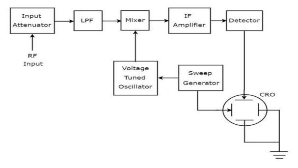
The **working** of superheterodyne spectrum analyzer is mentioned below.
