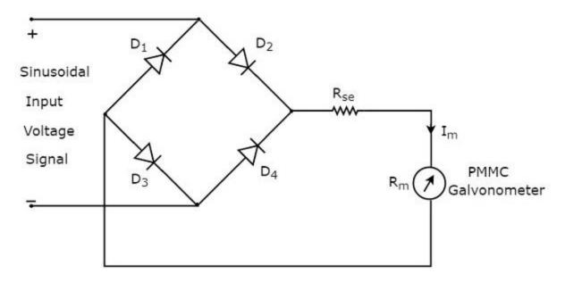
The **rms value** of sinusoidal (AC) input voltage signal is
