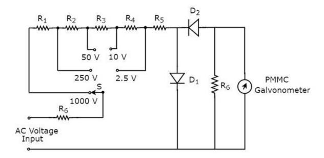
The above circuit looks like a **multi range AC voltmeter**. We know that, we will get AC voltmeter just by placing rectifier in series (cascade) with DC voltmeter. The above circuit was created just by placing the diodes combination and resistor,  $R_6$  in between resistor,  $R_5$  and PMMC galvanometer.
