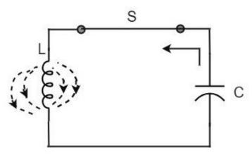
This continuation of charging and discharging results in alternating motion of electrons or an **oscillatory current**. The interchange of energy between L and C produce continuous **oscillations**.
