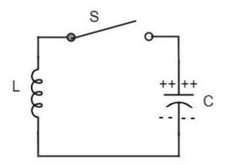
When the switch  $\mathbf{S}$  is closed, the capacitor discharges and the current flows through the inductor. Due to the inductive effect, the current builds up slowly towards a maximum value. Once the capacitor discharges completely, the magnetic field around the coil is maximum.
