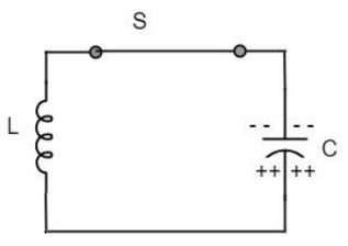
Once the capacitor is fully charged, it starts to discharge to build up a magnetic field around the coil, as shown in the following circuit diagram.
