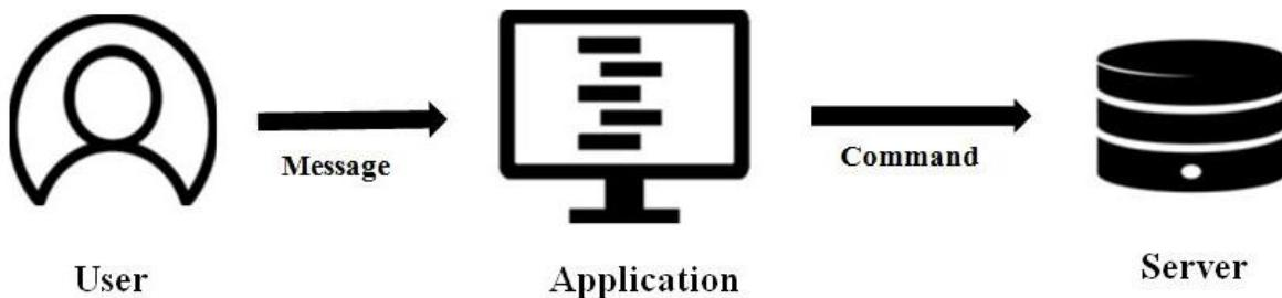
The user interacts with the view. The view generates an appropriate message based on the user's action. The update component receives this message and triggers a command.
