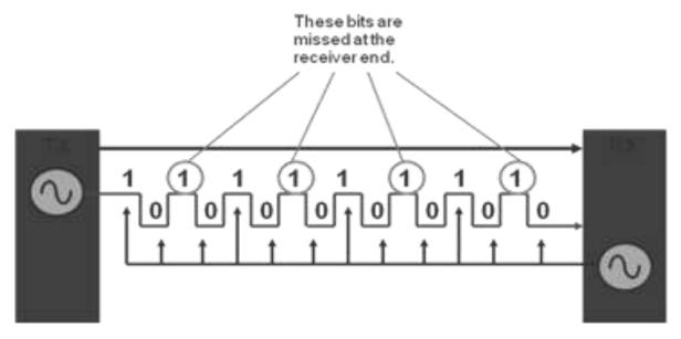
The data is transmitted at regular intervals. With timing derived from the transmitter's oscillator, the data is sampled at a faster rate than the transmitter. If the oscillator at the receiver end was running slower than that at the transmitter end the receiver would miss some of the bits of the transmitted signal.
