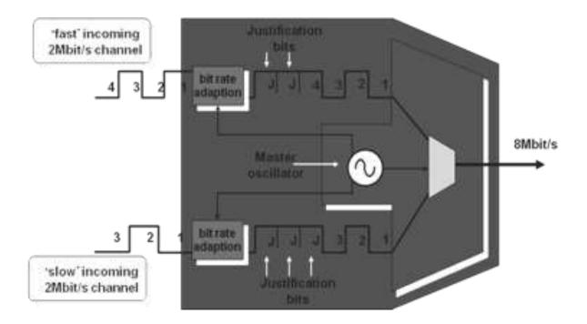
Justification bits are added to lower order signals so that they can be multiplexed at a single rate. The equipment oscillator is used as a timing source for the bit rate adaption process on the lower order and also on the multiplex proceed. Justification bits are discarded at the received end when the signals are de-multiplexed.
