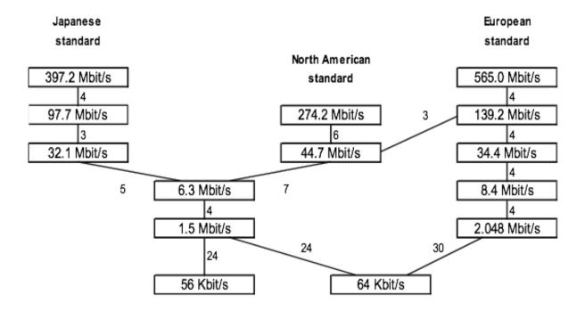
The higher bit rate links also require additional bits for framing and control. For example, an 8.4 Mbits signal comprises of  $4 \times 2.048$  Mbits = 8.192 Mbits, with the remaining 256 Kbits being used for framing and control.
