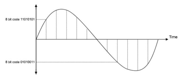
This comprises of 1 polarity bit with the remaining 7 bits used to identify the quantization level (as shown in the above figure).
