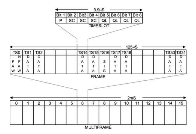
The duration of a multi-frame can be calculated using the following:
