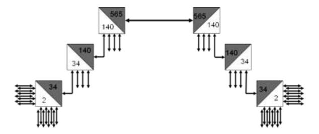
There also existed "jump" or "skip" muxes that would allow multiplexing of 16 2 M signals into a 34 M signal without the intermediate 8 M level.
