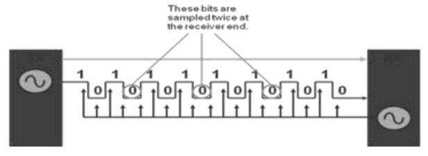
Or, if the receiver clock was running faster than that of the transmitter, the receiver would sample some of the bits twice.
