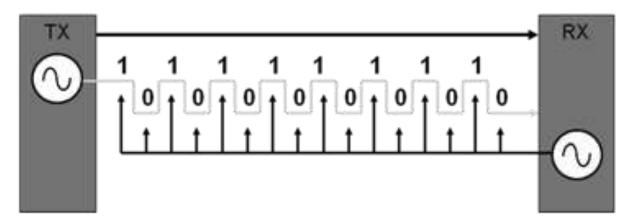
The data is transmitted at regular intervals. With timing derived from the transmitter's oscillator, the data is sampled at a slower rate than the transmitter. One of the disadvantages of PDH was that each element was synchronized independently. For data to be received correctly, the sampling rate at the receiver end must be the same as the transmission rate at the transmitter end.
