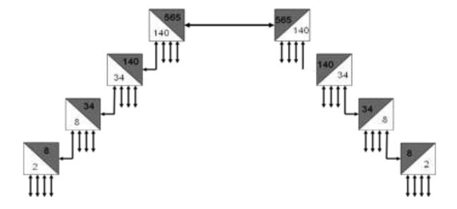
PDH technology allow successive multiplexing of a signal from 2 M - 8 M, from 8 M - 34 M, from 34 M - 140 M and finally 140 M - 565 M systems.
