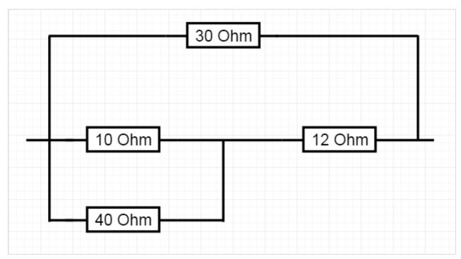
We have to find the equivalent resistance of this network. At first, we will try to get the result by hand, then try to see whether the result is matching with the prolog output or not.
